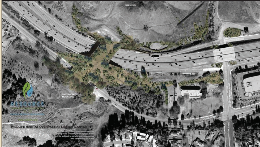
This plan calls for a 165-foot wide, and 200-foot long overpass that would cross the 10 lanes of the 101 Freeway at Liberty Canyon in Agoura Hills. The bridge would be covered in vegetation, making it more attractive for wildlife crossing between the Santa Monica Mountains and the Simi Hills according to the proposal released by the California Department of Transportation.
